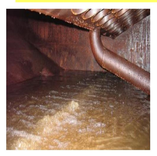
Air test into jigger in Tully C pan after operation for 15000 hours (during 4.5 seasons).
